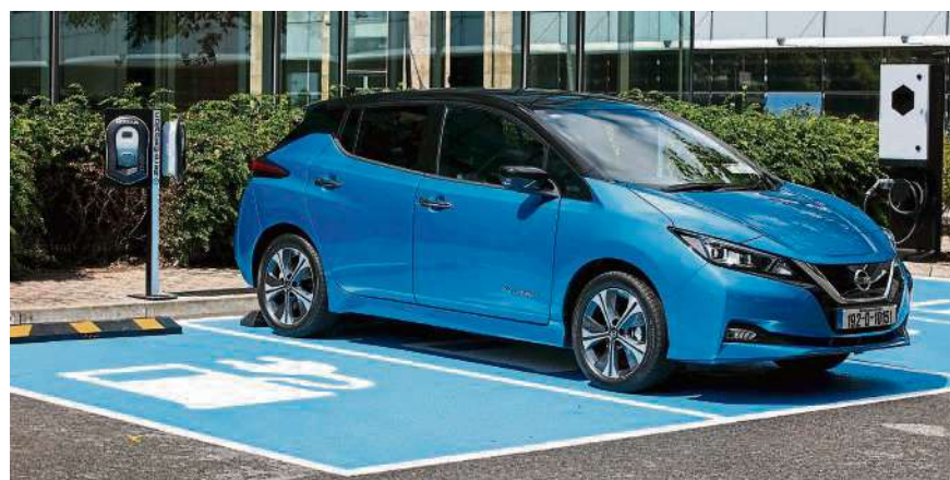
Nissan Leaf: The 62kWh variant offers up to 385kms on a single charge.
